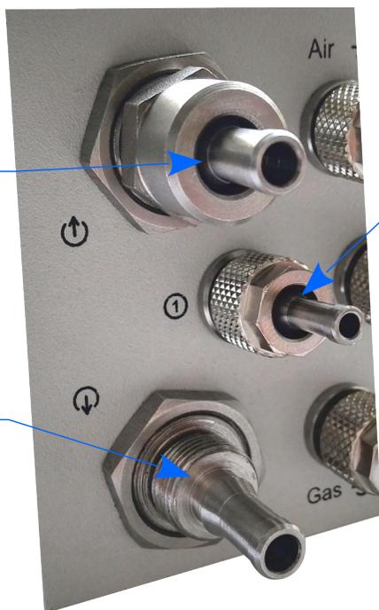
In High-pressure configuration, gas outlet is different than in standard version of mamos analyser. It is, similar to the dual-mode gas port. It allows to use standard silicone hose or PTFE tubing secured with a nut. This type of gas port allows for a secure, air-tight connection with a process (for both inlet and outlet).
