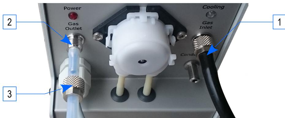
Gas ports in mamos, both in gas dryer and analyser are dual-mode, i.e. user can establish
