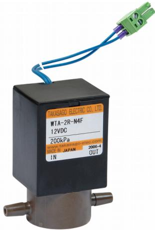
Gas sensors (of all types) for proper work require periodical ventilation with ambient air. Our on-line analyser handles ventilations automatically. Due to scheduled plan, analyser switches to source of fresh air with help of a solenoid valve. Since August 2015, 3-way solenoid valve was replaced with a pair of shut-off valves. In this, new configuration, one of the valves is always energised, while the other one is resting – this provides more stable heat distribution of mamos components.
