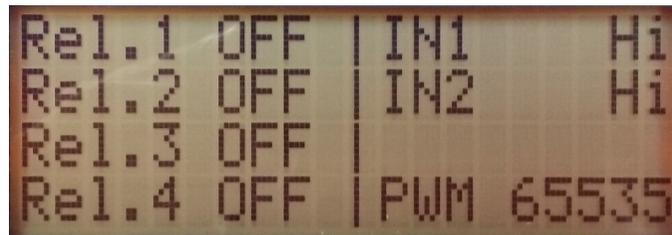
Screen with status of relays, digital inputs and PWM output.
