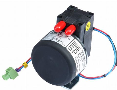
SP620 EC-BL - main gas pump in mamos analyser. This **diaphragm pump** is equipped with **brush-less motor**, that in comparison to a pump with traditional motor, is much more resistant to work in dusty environment. By default pump efficiency is set to give 1,5 l/min flow.
